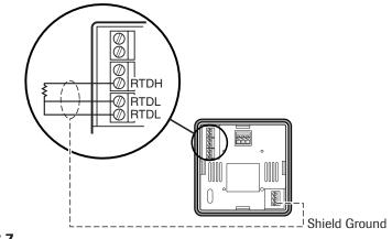
Figure 3.7 Three-Wire RTD Connections with Shield
